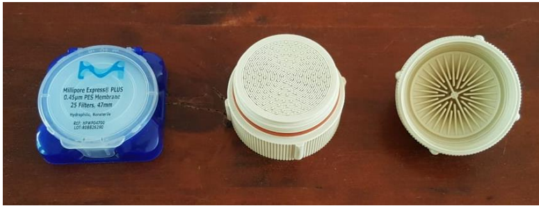
Links: Millipore Express Plus 0,45 µm PES membraan, 47mm Rechts: Swinnex filterhouder, 47 mm
