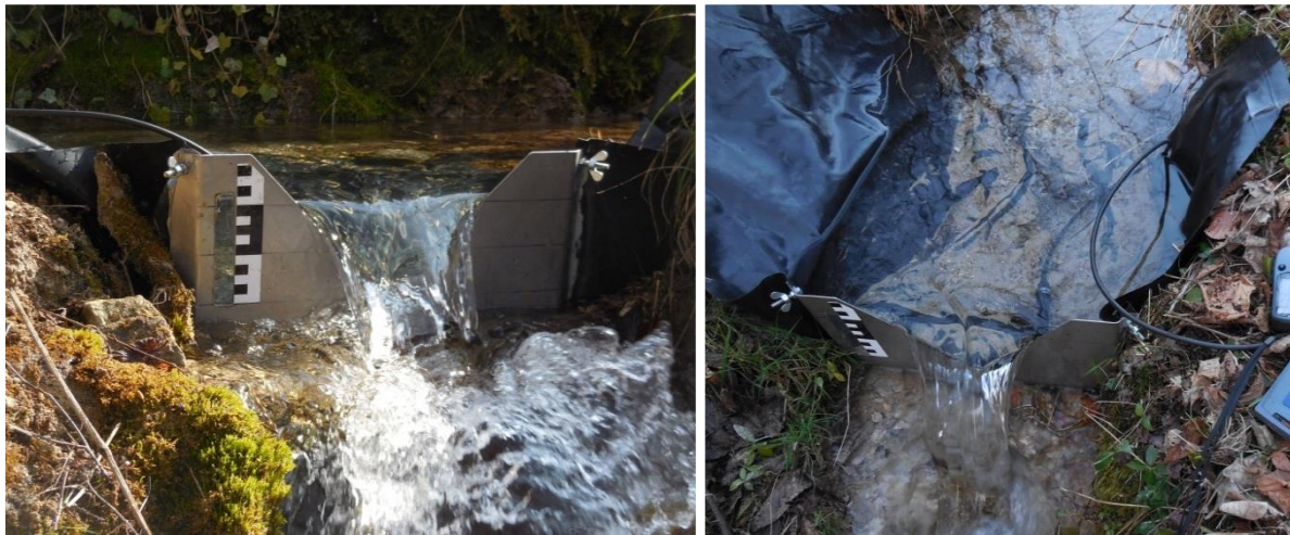
Figure 3.4: Small version of the portable sharp-crested weir (right) and from above (left) with plastic cloth
