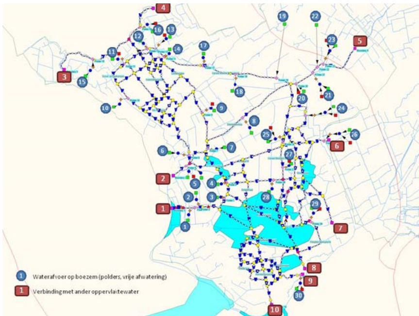
Fig. C1. A scheme of the SOBEK-model of National Park Weerribben-Wieden (between 52°48' N – 5°53' E and 52°38' N – 6°08' E). Small white circles are individual segments, red blocks and blue circles are boundary sites
